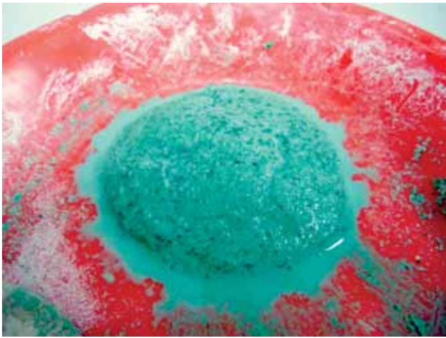
Egyptian Blue cake, made of malachite, quartz and other ingredients, prepared YSU Armenian Egyptology Centre before firing.
