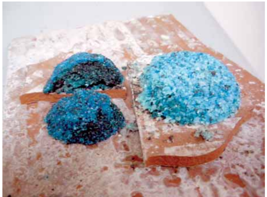
Egyptian Blue cakes after firing – note the different tones reflecting different proportions between constituents.
